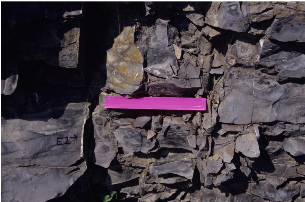
Figure 13g. ENE-striking fractures with calcite vein fills at the Borodino Reef in the Tully Formation. (Fractures range in strike from N76^{\circ}E to N60^{\circ}E ). (Locality 2 on photograph location map, Figure 13a). Photo by Jacobi.
