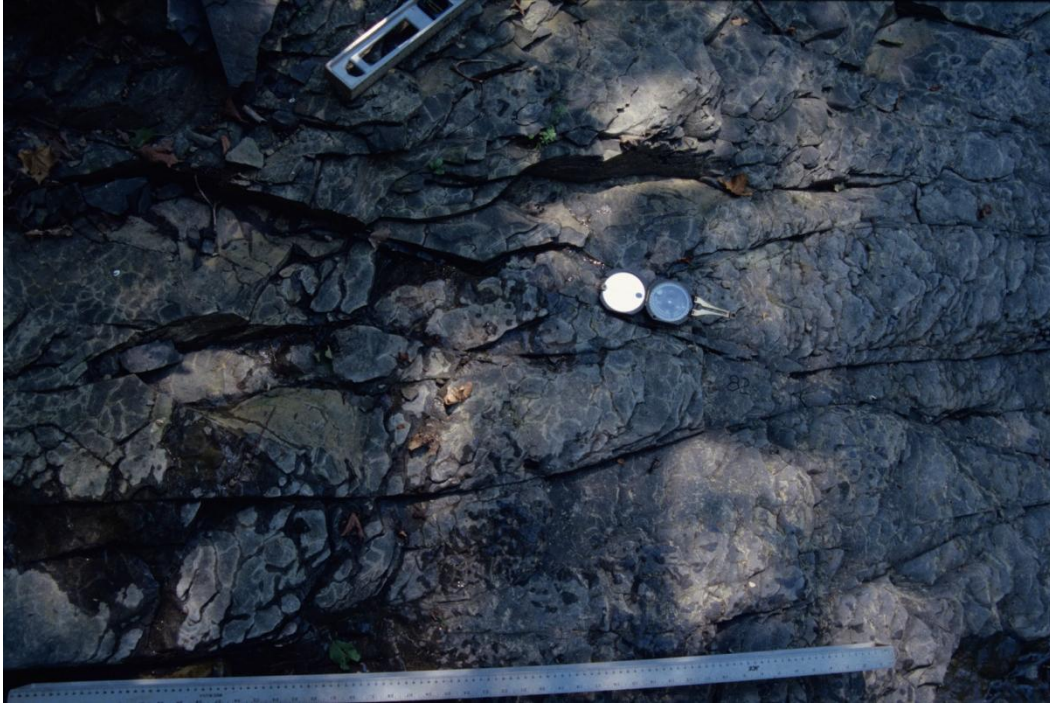
Figure 13h. Fracture intersection and interaction at Staghorn Point in the Genesee Group. The master (older) fracture strikes 343^{\circ} and the younger curving intersection fractures trend about 326^{\circ} . Photo looking down on outcrop. (Locality 3 on photograph location map, Figure 13a). Photo by Jacobi.
