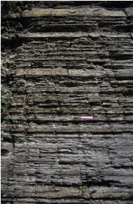
Figure 13m. Larger view of the vertical outcrop in the Genesee Group at Fillmore Glen (about 5 km south of the central study area) shown in Figures 13k and l. The dominant fractures/faults strike NNW ( 340^{\circ} ). Ruler is 15 cm long and in same position as in the preceding two figures. Photo by Jacobi.
