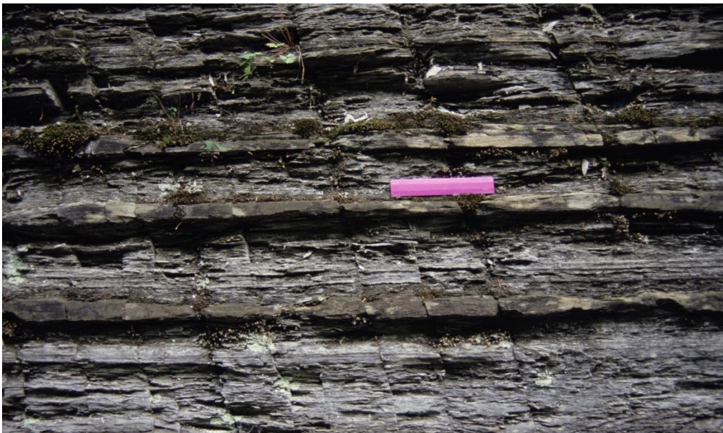
Figure 13k. Fracture intensification in the Genesee Group at Fillmore Glen (about 5 km south of the central study area). The dominant fractures strike strike NNW ( 340^{\circ} ). Photo looking at cliff. Ruler is 15 cm long. A small amount of offset occurs on each fracture, as seen in Figure 13l. Photo by Jacobi.
