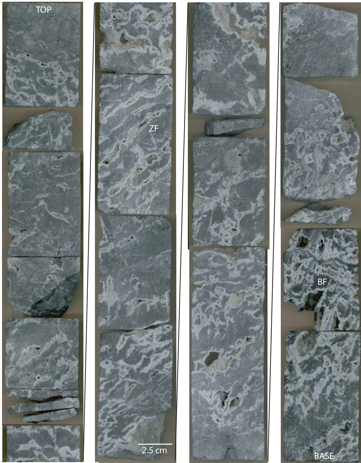
Figure 11. Core photographs from Whiteman #1 well, Chemung County, NY. This core has common fractures, vugs, zebra fabrics (ZF), boxwork fabric (BF) and an overall brecciated appearance. White saddle dolomite lines vugs and fractures in gray matrix dolomite. Core is 5cm (2 inches) wide.
