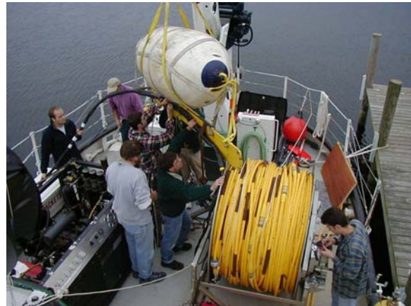
Figure 3. Seismic streamer on reel on aft deck.
