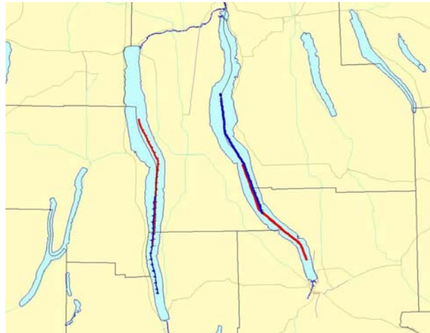
Figure 4. Four seismic tracklines on Seneca and Cayuga lakes (see Appendix also).
