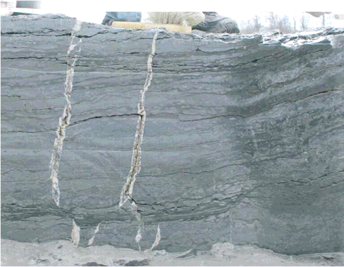
Figure 37 - Fractures change dip direction when crossing shaly bed taken from eastern wall of Trench 4, body two lies to the left)
