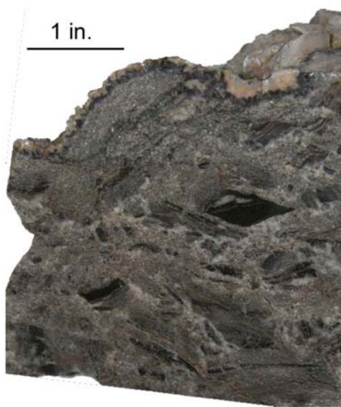
Figure 30 – Cross-section of a brecciated block from inside dolomite body
