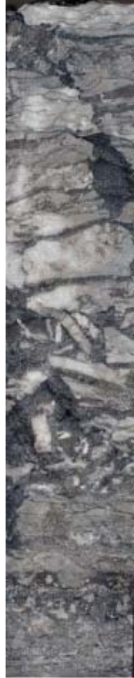
Figure 23 – Fault breccia (from Hole 4: 14 ft.)
