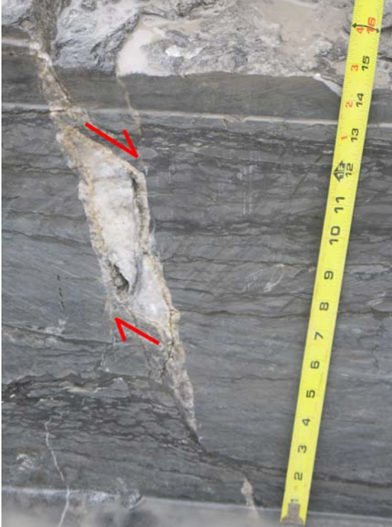
Figure 38 - Rhombohedral pull-apart with red arrow to indicate motion direction (taken from eastern wall of trench 6)
