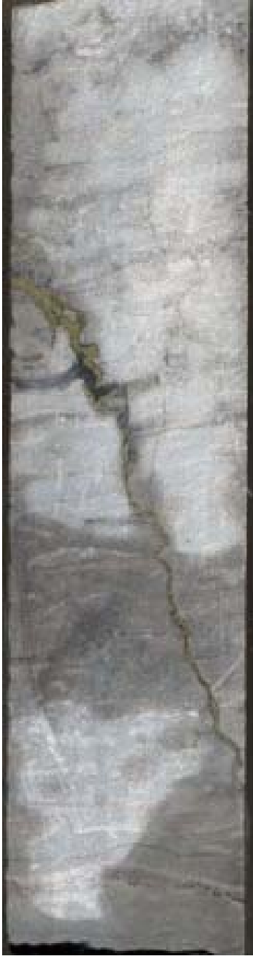
Figure 21 – Fracture filled with pyrite and bitumen (from Hole 1: 23 ft.)
