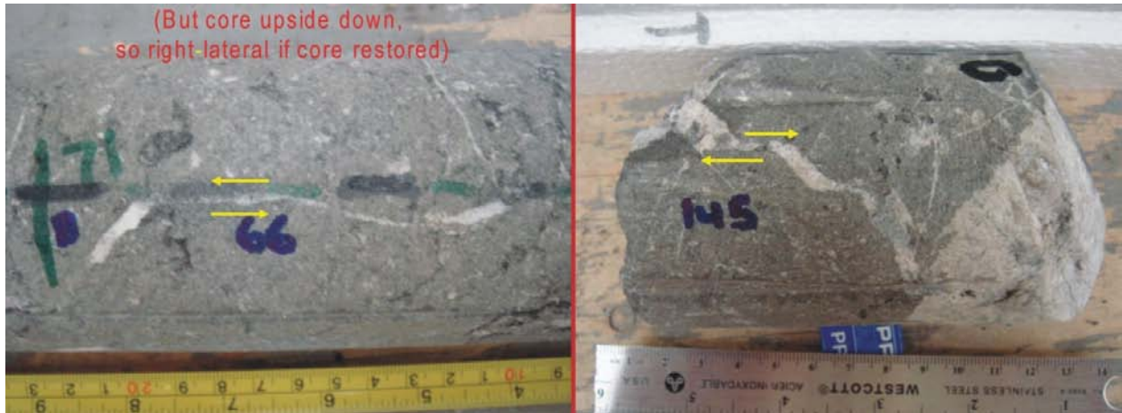
Figure 19. Example of rhombochasm (releasing bend) geometries that indicate sense of incipient motion from the Schwingel #2 horizontal core. From Jacobi et al. (2007).
