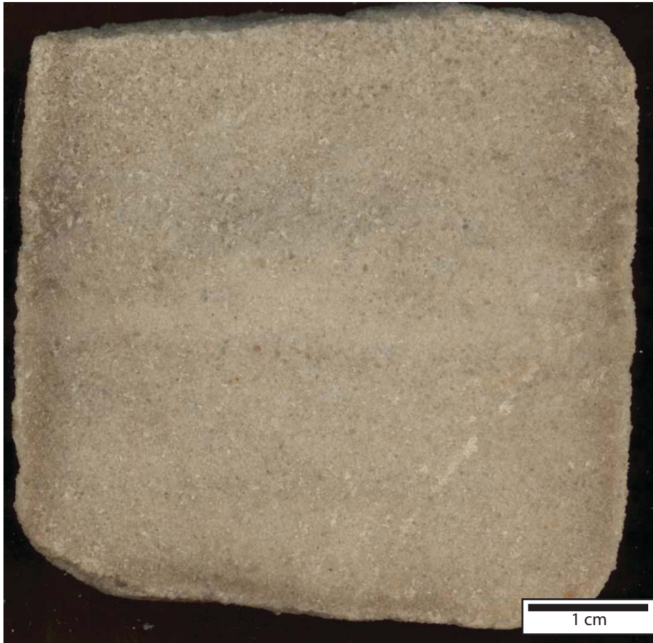
Figure 13. Core slab photo of cross-bedded Rose Run Sandstone from Kennedy #1 well.
