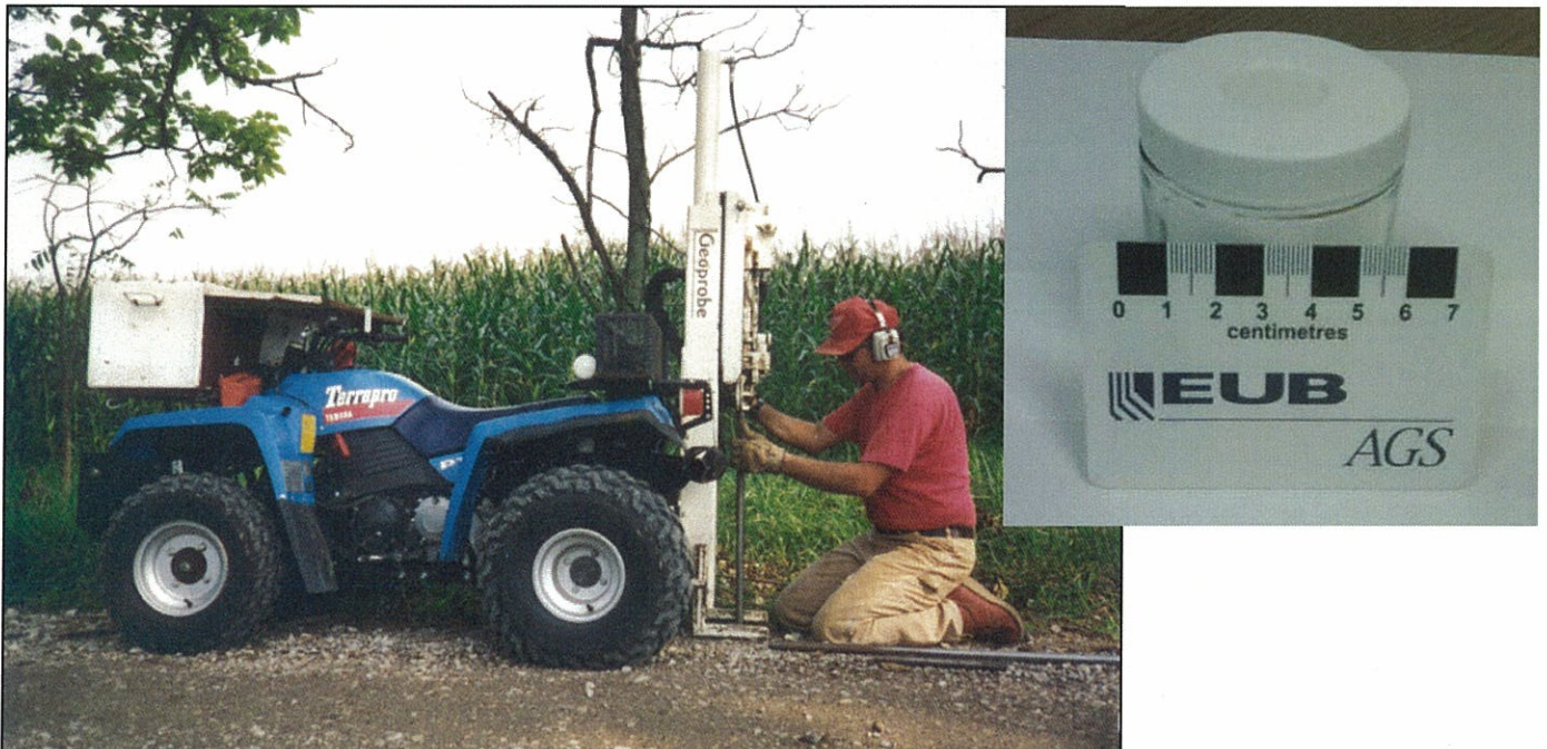
Figure 6. An ATV-mounted Geoprobe was used to collect soil cores from 8-foot depth and soils were stored in 4-ounce glass jars with Teflon septa plastic lids for transport to the laboratory in Golden, Colorado.
