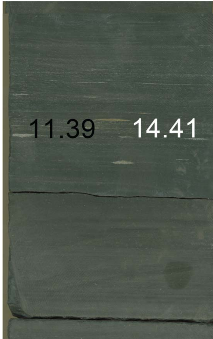
Figure 27. Laminations and lenticular bedding in organic- and carbonate-rich shale. Black number is TOC content and white number is percent carbonate. Lighter colored grains are fossils made of calcium carbonate. Core is 2.5 inches across.
