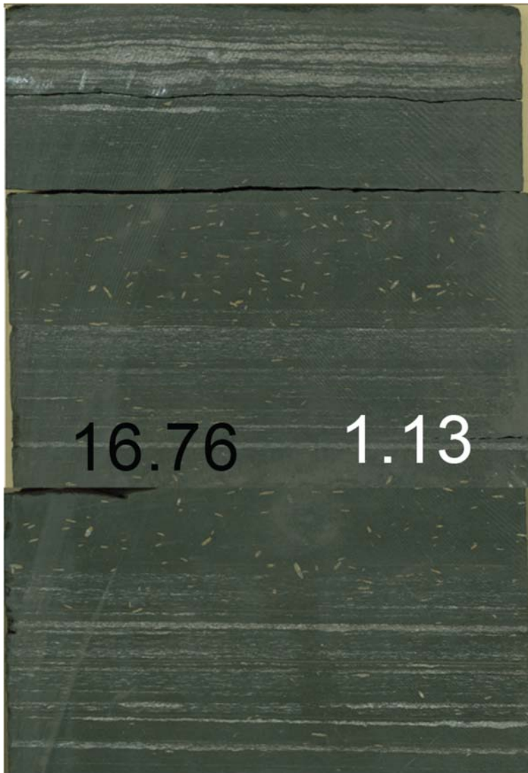
Figure 28. Intervals of laminations interbedded with intervals of randomly oriented fossil debris (lighter colored). There are two distinct intervals of chaotic bedding that could be storm beds composed of the material that is present in the laminated facies. Core is 2.5 inches across.
