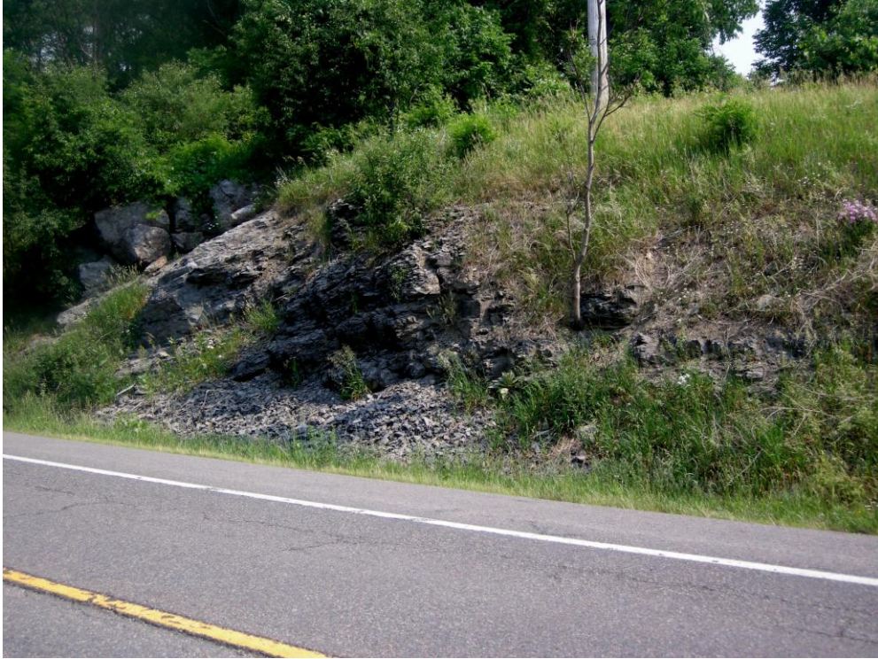
Figure 41 Inclined Strata Oriented 175^{\circ}/30^{\circ} in the Tully Limestone at Station SPA-2
