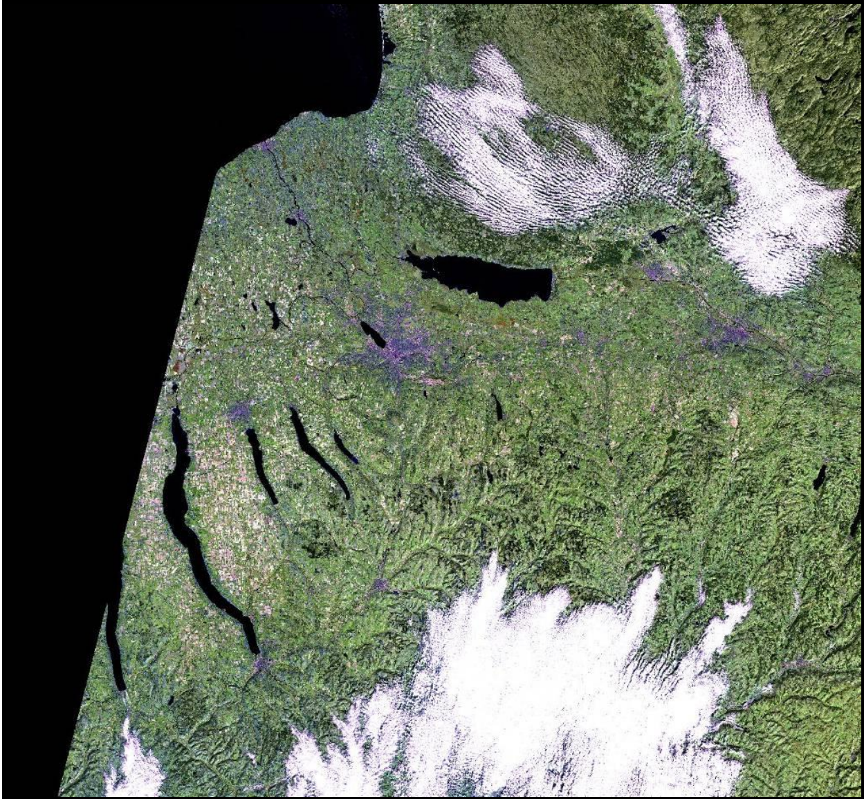
Figure 22 Landsat 7 Color Composite of Channels TM7, 5 and 2 in Red, Green and Blue.
