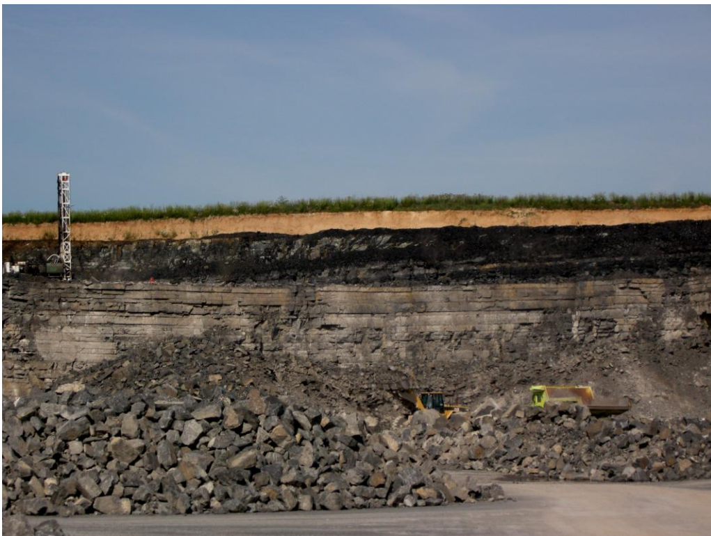
Figure 14 Contact Between the Gray Onondaga Limestone and the Overlying Black Marcellus Shale at Station ROM-1 (See Figure 13 for Location).
