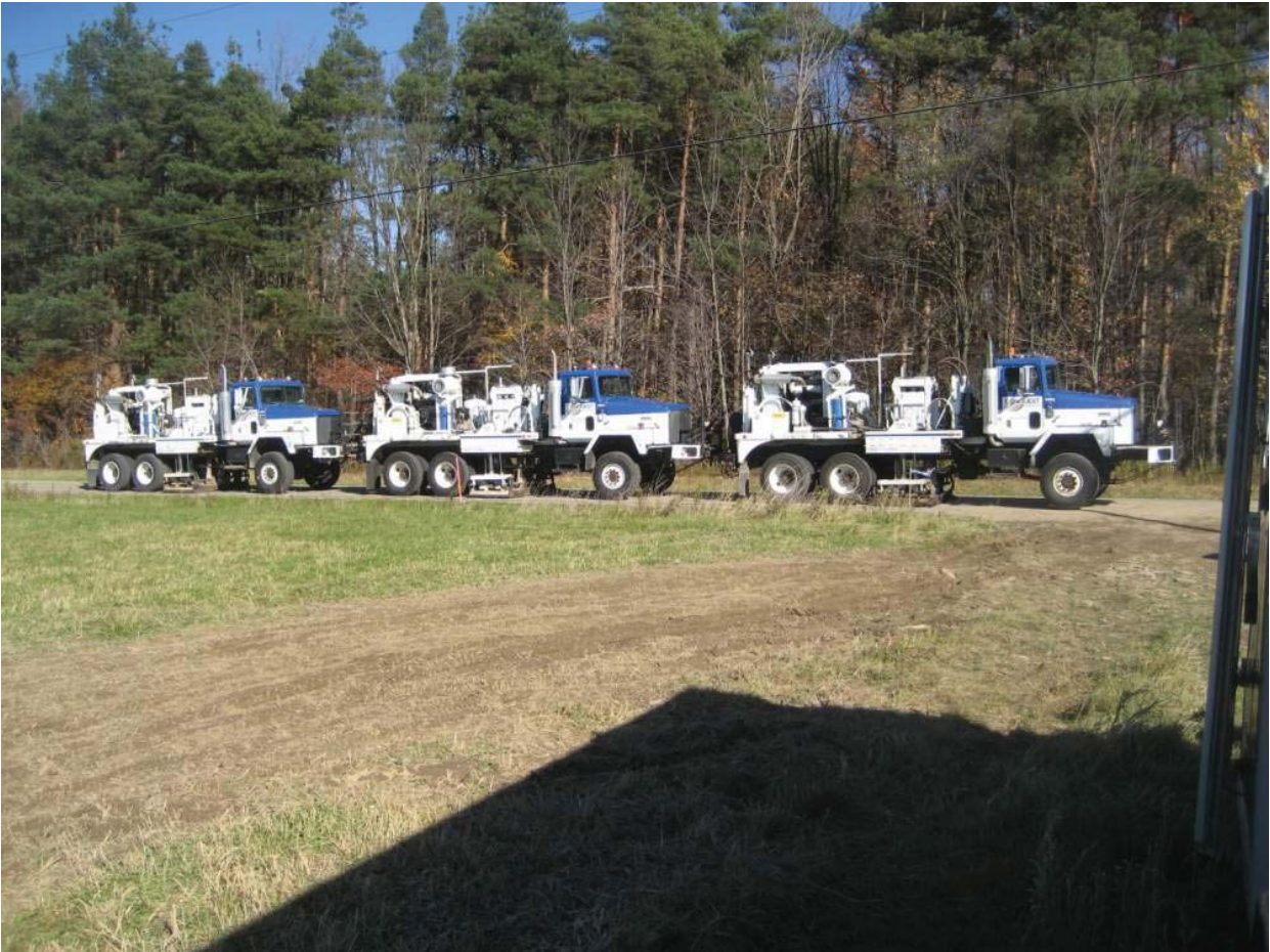
Figure 11: View of prospect area with vibrator trucks
