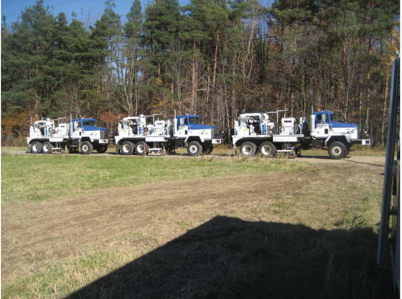
Figure A.12 - View of prospect area with vibrators
