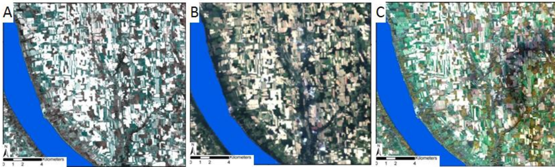
Figure 6.4,5&6-28. True color Landsat color composite; band combination R(3), G(2), B(1) for Grid 1. (A) image acquired April 28 th 2001, (B) image acquired June 15 th 2001, and (C) image acquired October 16 th 1999. Figure from Zelazny et al. (2010) and Zelazny (2011).
