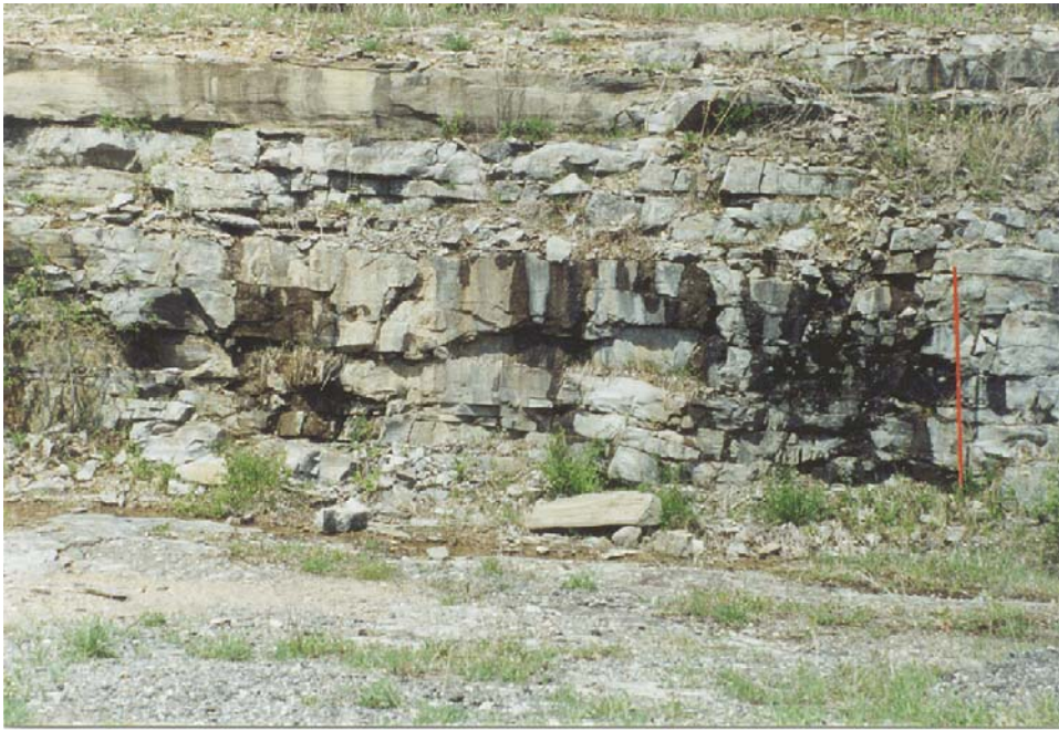
Figure 5-6 Cross Section of the Oxford Dolostone Northeast of Champlain, NY (Station CH-2). Note the Massive, Undulating Layers.
