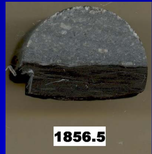
Core plug scan with break in shale
