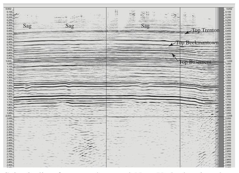
Seismic line from south-central New York showing three sags that have been drilled and produced gas from hydrothermal dolomite in Black River - These very subtle features are interpreted to be negative flower structures (courtesy of Fortuna Energy)
