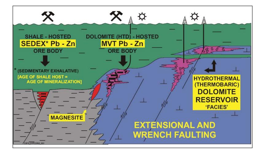
Hydrothermally altered carbonate reservoirs share much in common with carbonate-hosted MVT ore deposits and SEDEX deposits - they are all fault-controlled - timing of emplacement can in some cases be tied to SEDEX deposits
