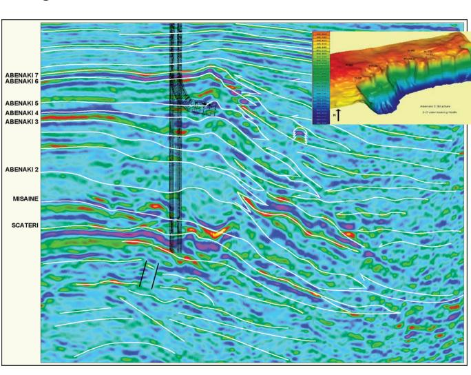
Seismic line over faulted hydrothermally altered Jurassic Abenaki margin, offshore Nova Scotia (from Encana)
