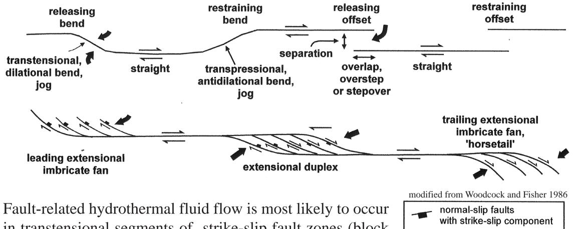
in transtensional segments of strike-slip fault zones (block reverse or thrust arrows). Even in overall extensional settings, upward fluid flow is most likely to occur where there is a component of strike-slip that opens a conduit to greater depth.
