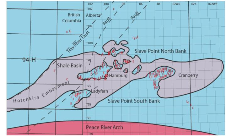
Ladyfern and several other Slave Point Fields occur where faults intersect fault-controlled margin active during Slave Point time
