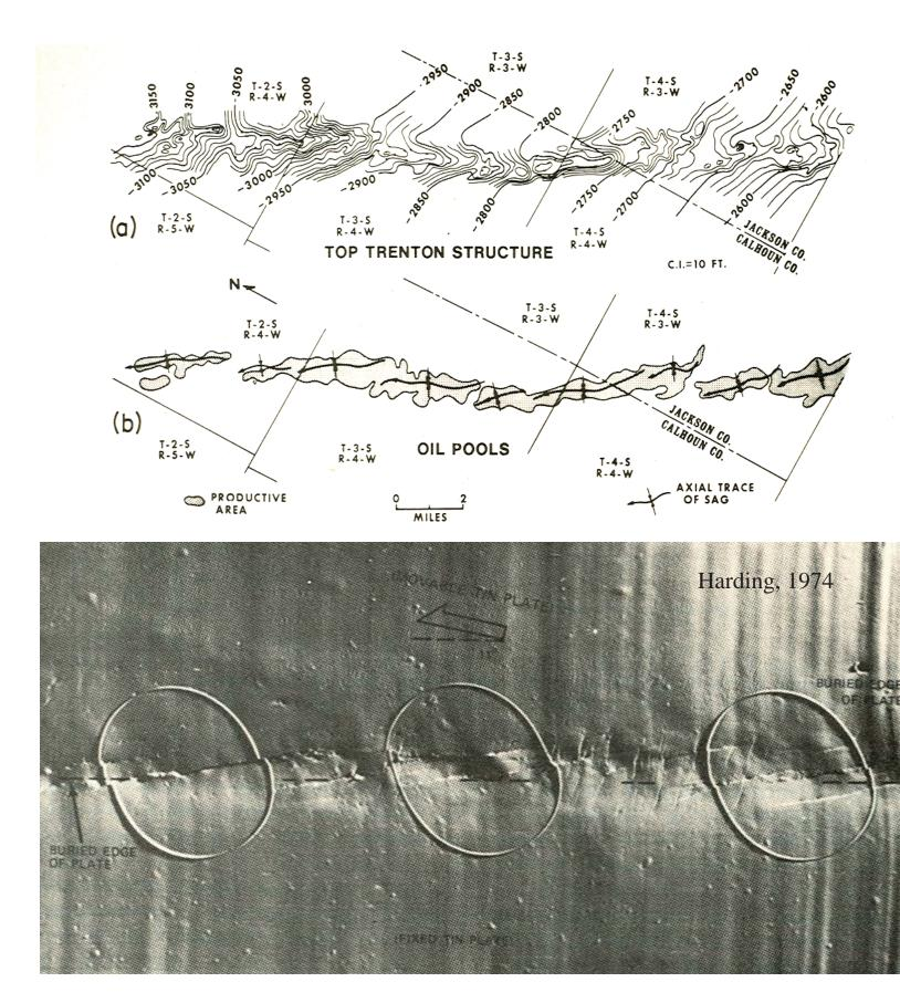
Harding (1974) modeled en echelon sags found in Albion Scipio Field (top) and found that they could only be produced by adding a component of extension to dominat left-lateral strike-slip motion
