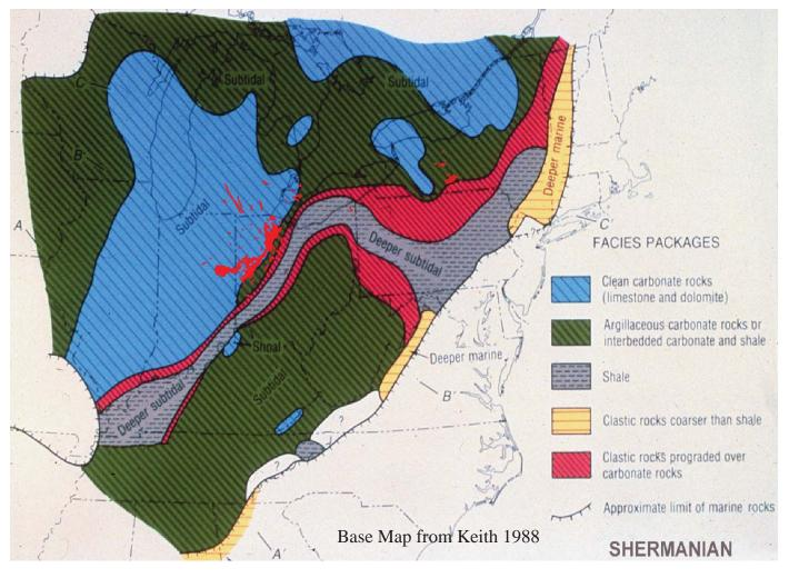
Many Trenton Black River Fields of E. North America (red) line up along margin-bounding faults active during Trenton time. Intersections with intraplatform faults best.
