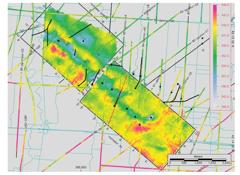
Time-structure map of the top Trenton Formation at Rochester Field in Ontario - note location of oil wells in en echelon sags - it is here that hydrothermal dolomite and hydrocarbons are found (courtesy of Talisman Energy)
