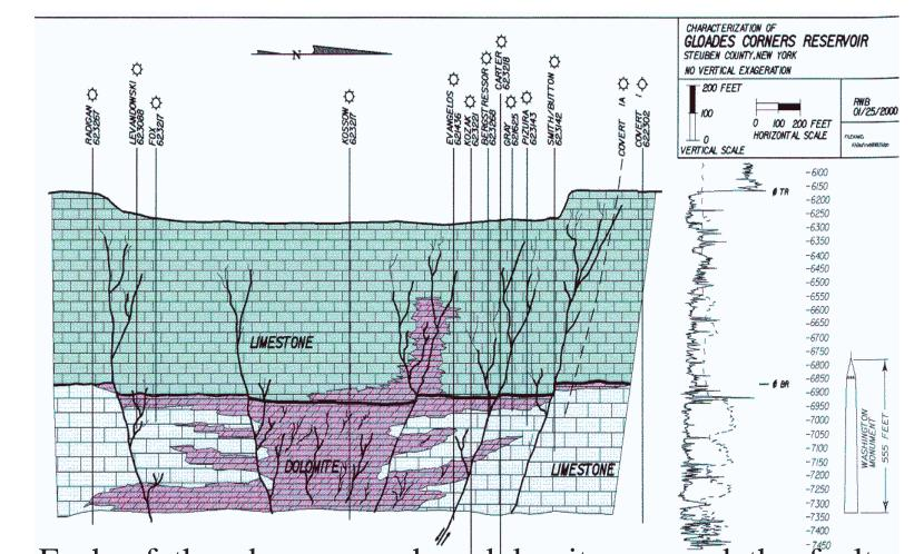
Each of the above sags has dolomite arround the faults (particularly on downthrown side) and limestone away from faults (figure from Columbia Natural Resources)
