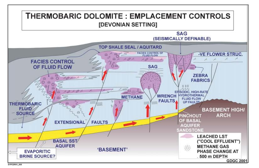
Structural settings for hydrothermal alteration - faultcontrolled margins and intraplatform wrench faults are most common sites
