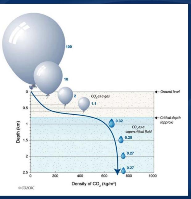
The density of CO<sub>2</sub> "tops out" at approximately 700 kg/mg<sup>3</sup> (43.7 lbs/ft<sup>3</sup>). This occurs at a depth of approximately 2.5km, or 8,200 feet. Since the Upper Logan Canyon occurs at or below that depth, a density 43.7 lbs/ft<sup>3</sup> was used in all capacity equations.
